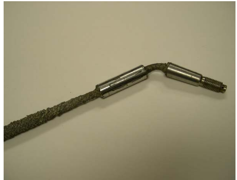
Stray Current Corrosion
